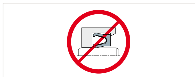
Fig. 4.34 – Incorrect installation in step-cut groove.
